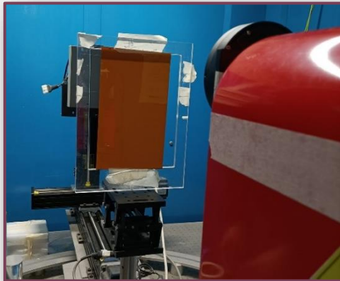
GafChromic™ XR-QA2 film calibrated at 80 kV
