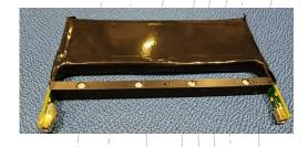
Two **scintillator** tiles (12 cm x 4 cm), placed upstream and downstream of the drift tubes pack, instrumented with SiPM
