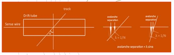
Space charge, attachment and recombination effects affect the experimental cluster counting efficiency
