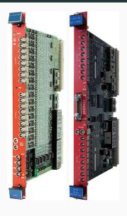
The readout system was based on custom differential discriminators developed at INFN Torino, commercial QDC (Caen v965) and commercial TDC (Caen v1290). The problem of this architecture is due to the QDC conversion time of about 10  $\mu s$ , that limits the event rate ( $L_0$  trigger) around 100 kHz. The current requirement, for Run 3, is the capability to sustain an event rate of roughly 5 M event/s.
