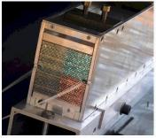
The Zero Degree Calorimeters (ZDC) feature a set of calorimeters placed on both sides of the interaction point, at about 113 m. The purpose is to detect spectator nucleons in order to determine the overlap region in nucleus-nucleus collisions.
