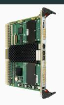
The FPGA carrier is the commercial loxos ifc1211 that has a 6  $\,\mathrm{U}$  VME format with a PowerPC processor, a Xilinx UltraScale FPGA and many other interface ports among which two FMC.
